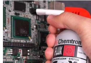
*Clean PCB after reworking, especially if using Soder-Wick Rosin*
